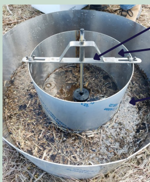
The bridge holding the measuring rod with float
